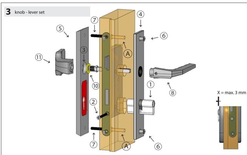
To install the handle for entrance door fittings: place the washer (10) over the square spindle (3), push the spindle through the exterior plate (5) then screw into base of handle and tighten.
