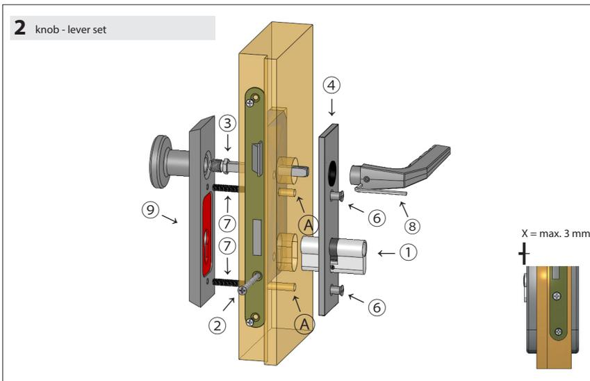
Place the inner fixing plate over the profile cylinder and spindle and fix it with the handle to mark the position of the screw holes on the door.
